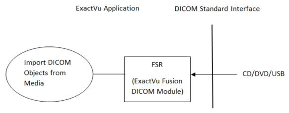
Figure 2: DICOM File-Set Reader Flow Diagram
